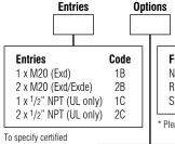
plug, suffix appropriate code with 'P', e.g. 2BP is 2 x M20 entries with one certified plug.
