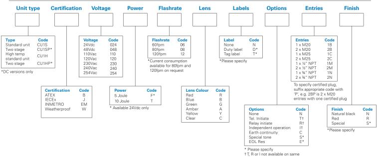
High temperature CU1H is set to 107dB(A). For the 24Vdc version 960mA @ 10J &750mA @ 5J
